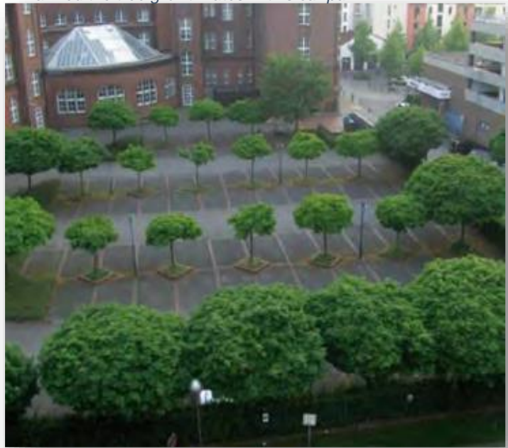
Figure 42 - Lack of soil volume and compaction has harmed the tree growth rates in this car park
